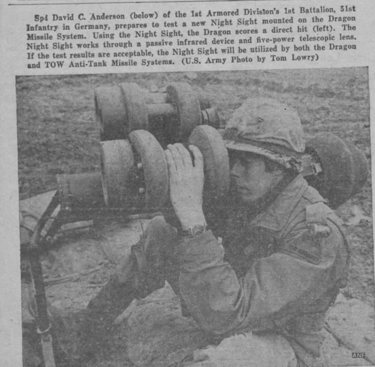
Sp4 David C. Anderson (below) of the 1st Armored Division's 1st Battalion, 51st Infantry in Germany, prepares to test a new Night Sight mounted on the Dragon Missile System. Using the Night Sight, the Dragon scores a direct hit (left). The Night Sight works through a passive infrared device and five-power telescopic lens. If the test results are acceptable, the Night Sight will be utilized by both the Dragon and TOW Anti-Tank Missile Systems. (U.S. Army Photo by Tom Lowry)
