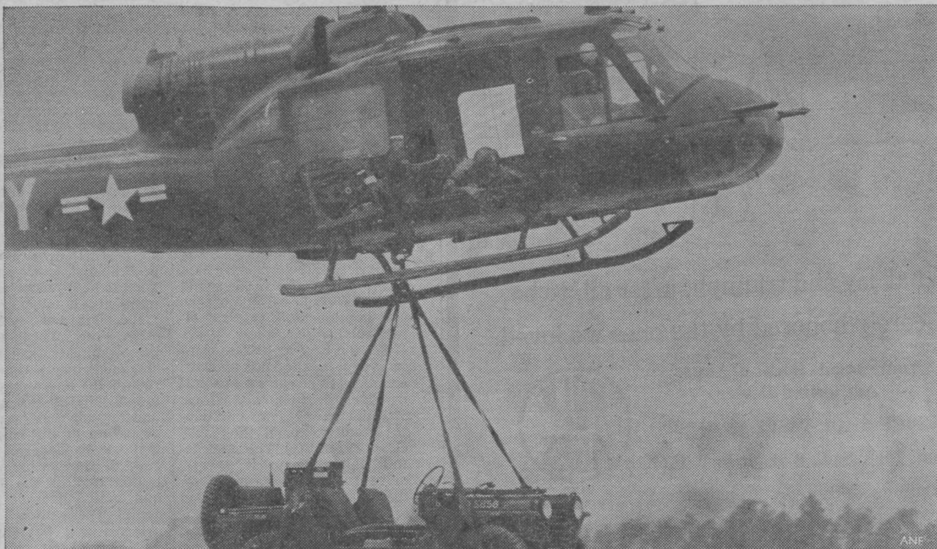
SHOCK TREATMENT — Jeep-mounted radio equipment gets the "once over" from an airborne rigging specialist during the air transportability phase of a service test conducted at Fort Bragg, N.C., by the Airborne, Electronics and Special Warfare Board. The board is an activity of the U.S. Army Test and has Evaluation Command. Purpose of the test is to determine what effects air transport has on radio equipment.
