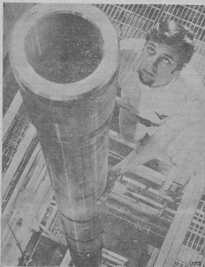
DOWN THE HATCH — A technician keeps a watchful eye on the 35-foot long 175mm gun tube as it descends into a high fluid pressure pit at the U.S. Army Weapons Com- mand's Watervliet Arsenal, Watervliet, N.Y. The pressure process will nearly double the in-service life of the tube.
