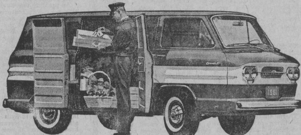
CORVAIR—Side doors open a full 49" wide. Loading height is a low 14" DMI
