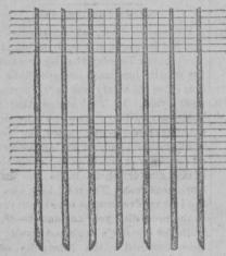
REVETMENT FOR PROTECTING RIVER BANK. stead of perpendicular and to keep it covered with vegetation. The willow is admirably adapted to holding alluvial soil in place. It is far more serviceable for this purpose than walls of masonry, and the facility with which it reproduces itself by seed, suckers, sprouts and cuttings, both natural and artificial, makes its use very simple and inexpensive.
