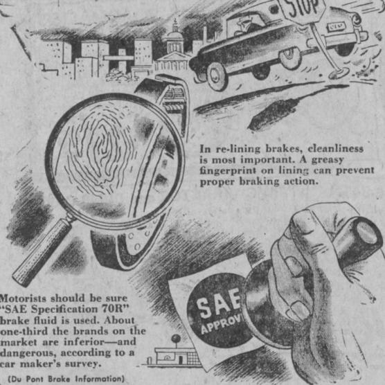
In re-lining brakes, cleanliness is most important. A greasy fingerprint on lining can prevent proper braking action.
