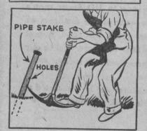
You can save time and energy in pulling pipe stakes with the method shown above. Stakes used to anchor various farm machinery firmly to the ground may be moved easily by getting proper leverage with a pick, in the manner above. Holes drilled in each stake to take the pointed end of the pick are helpful, too.
