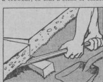
filling can be placed underneath. If the sidewalk is one continuous strip, the sunken part should be broken into small pieces, to be packed and used as a foundation for a new layer of concrete. If you are not familiar with the work, it might be a difficult job, but one that a concrete contractor would find very simple.
