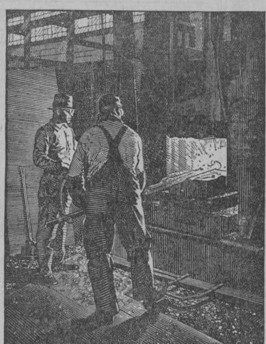
A scene in Chevrolet's great drop forge plant. A front axle is being forged from a bar of fine alloy ste
