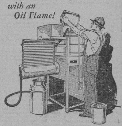
PREVENT spoilage, end rejections, make bigger profits by chilling milk with the wonderful new Superfex Oil-Burning Milk Chiller. Just burning a few cents' worth of kerosene creates sufficient icy cold for cooling 20 to 30 gallons (larger size 25 to 45 gallons) from animal temperature to 40° as fast as drawn! Insulated storage box for keeping chilled milk well below 50° until shipping time easily built from specifications furnished free
