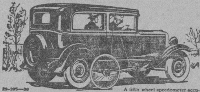
A fifth wheel speedometer accurately measures speed and mileage on all Chevrolet test runs at the Proving Ground.
