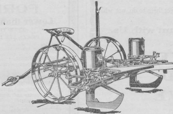
Plant accurately whether set for checking, drilling or power drop. Without stopping the team the variable clutch can be set to plant 2, 3, or 4 kernels to the hill. Edge, flat and full hill plates interchange in the same hopper. The automatic marker requires no attention.
