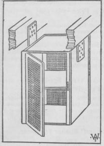
A useful device, known as the hanging cellar cupboard, can be made from an ordinary store box, a pair of hinges and two small pieces of fly screen, the entire cost not exceeding 60 cents. Two sides of the box are covered with netting, one side being in the form of a door. Some of the boards removed from the box are used to form the frame of the door, while the remainder will form the shelf and supports When completed the outfit is suspended to the joists at a convenient place in the cellar.
