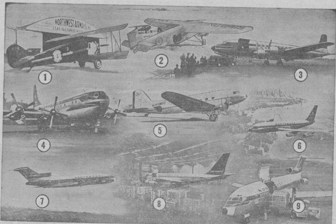
NORTHWEST AIRLINES aircraft in use over 40 years of the company's history illustrate the development of aviation: (1) Sison Detroiter, which went into service in 1926, carried three passengers at 85 mph. (2) Ford Tri-Motor, 1928, cruised at 125 mph with 16 passengers. (3) DC-6B, 1953, carried 64-76 passengers at 315 mph, also provided all-cargo version (pictured). (4) Boeing double-decked Stratocruiser, 1949, accommodated 83 luxury passengers, cruised at 320 mph. (5) DC-3, late 1930's, 21 passengers, 185 mph. (6) 720B fan-jet, 1961, 623 mph maximum, 111 passengers. (7) 727 fan-jet, 1965, 93 passengers at 607 mph. (8) 707-320 fan-jet, 1963, 112-165 passengers, 585 mph cruising speed over 6,000-mile range, providing maximum cargo as well as passenger lift. (9) 727C fan-jet, 1966, convertible passenger-cargo airline, same specifications as 727, but offering big-door cargo capacity, to bring jet-age cargo service to smaller cities. Northwest, which began operations on an air mail route linking Minneapolis-St. Paul and Chicago and now serves routes spanning the U.S. and the Pacific, notes its 40th anniversary October 1, 1966.
