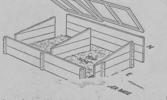
Anyone handy with a hammer and saw can construct this sturdy seed frame. It is made up of four sides, and a hinged top glazed with Vimlite, flexible plastic glazing. Vimlite is used because it is shatterproof, lightweight, has good insulation qualities and is easy to install. No grooving of the frame, or putting in necessary. Vimlite is merely tacked in place like fly screen.
