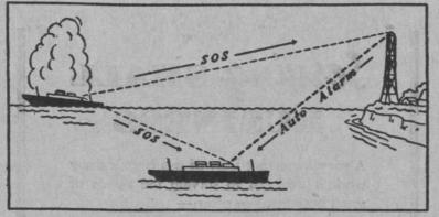
In the above illustration is shown how the radio auto-alarm might func tion. The ship in the distance is in trouble and sends the SOS distress signal. It is assumed that the radio operator on the nearer ship is not listening at the moment, however, the shore station picks up the signal and resends it after sounding the auto-alarm which brings to attention the radio operator on the inbound vessel.
