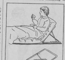
SAVES LIFTING OF PATIENT. two parallel ratchet rods having downbraces. Hinged to the rachet rods is the adjustable framework section of the mattress, to which arms are pivoted, the free ends of which engage and
